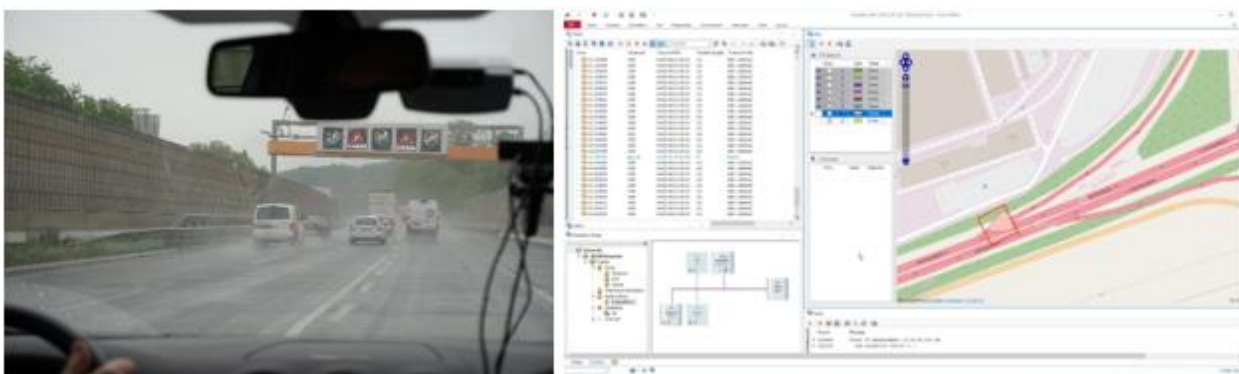
Figure 69 – The VMS (a) and the C-ITS RSUs (b) send the new C-ITS messages for mixed traffic control
