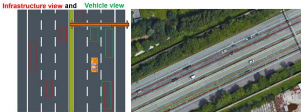
Figure 50 – Combined infrastructure (red) and vehicle (green) view (a) and generated anonymised vehicle trajectories on the real test-site (b)
