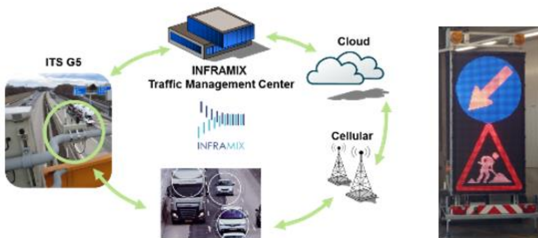
Figure 51 – INFRAMIX hybrid communication model (a) and intelligent roadworks trailer (b)
