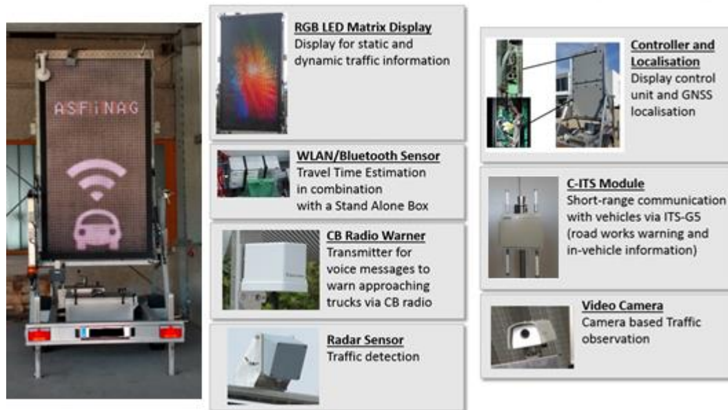
Figure 67 – IMIS trailer displaying the INFRAMIX SC1 sign (left) and IMIS components (right)
