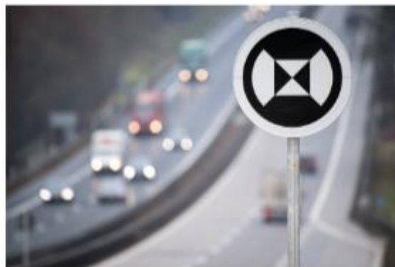
Figure 17– German sign for positional calibration of AVs
