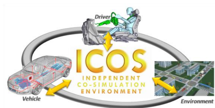
Figure 5 – Interdisciplinary modelling of the vehicle, including driving behaviour and environment
